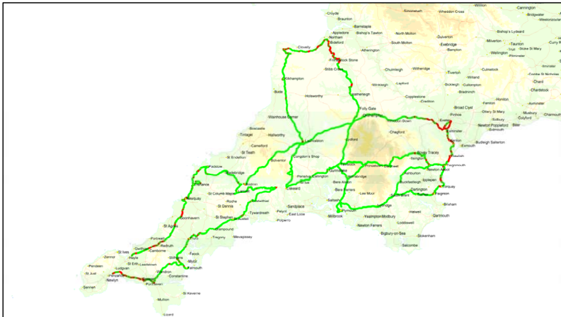
Measured daytime audio quality of DRM (64 QAM) from Plymouth on 855 kHz (green – good; red – bad)
