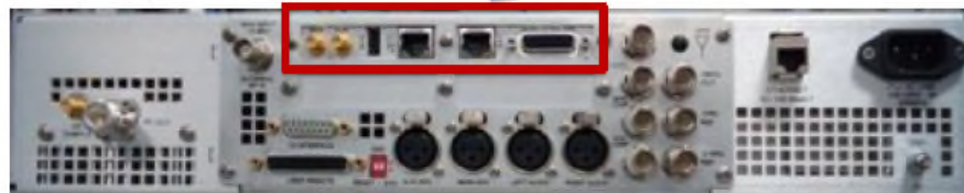
GatesAir Dig. Modulator Card Installed in Flexiva FM Exciter
