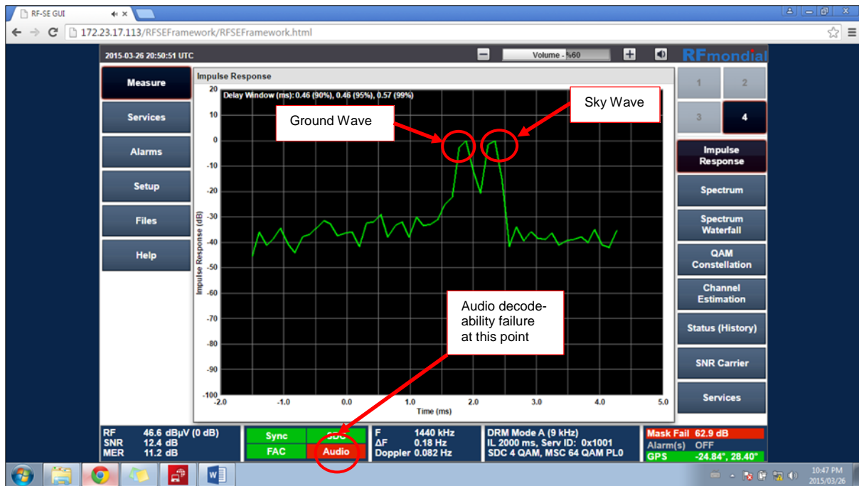
Figure 5: Broadcom antenna. Impulse response indicating the fading zone.
