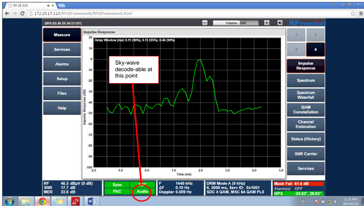
Figure 6: Broadcom antenna. Impulse response indicating that the sky wave is dominant.
