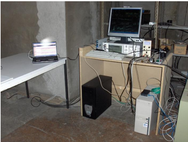
FIGURE 5 DRM generator, modulator and exciter
