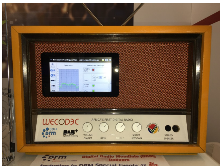
Our community-built DRM/DAB Multi-Standard Digital Receiver with DRM, DAB+ and FM function (DRM30 and AM were still under development), demonstrated and awarded in September 2017 at IBC in Amsterdam.
