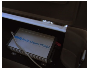
DC/AC Inverter to supply 230V
