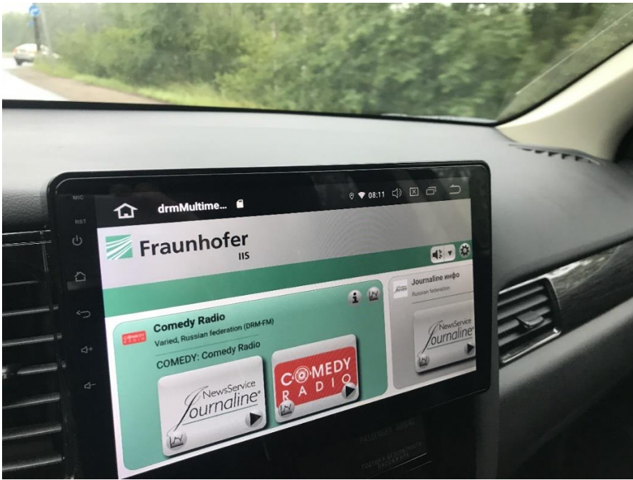
Figure 8b: Fraunhofer DRM MultimediaPlayer Radio App software was installed in Mitsubishi Outlander measuring vehicle's Android-based radio set with an external FM receiver dongle connected via USB
